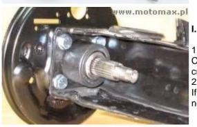
Completely disassemble the trailing arm hub assembly. Check the trailing arm for damage or cracks. If damaged or cracked, repair or replace trailing arm.
