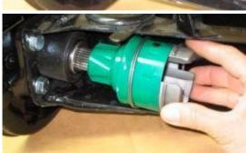
3. Install the tripod housing on to the splined portion of the stub axle. You may have to tap it on with a hammer. Leave the wire ring on the tripod housing, you will need it later.
