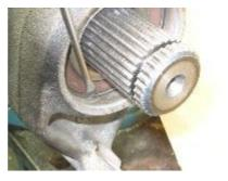
13. Push in the axle into the bearing. Check and correct the bearing position in the bracket body.
