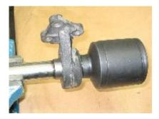
15. Grease splines with a graphite grease and push in the joint onto the axle up to resistance.
