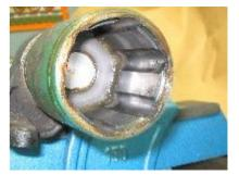
5. Remove the grease from the joint.6. Fix the axle with joint in a vice..
