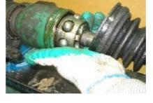
4. Pull out the internal joint elements.
