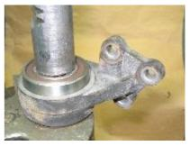
11. Push in the new bearing into the bracket.
